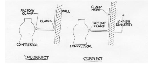
Piping attached to a vibrating object (such as a compressor, or compressor base) must be supported in such a manner that it will not restrict the movement of the vibrating object. Rigid mounting, as shown below, will fatigue the tubing. When a reduced riser is necessary, reduce the pipe on the high side of the riser only. A reduction of the low side backs up a large quantity of oil on the horizontal pipe run, not in the trap.
