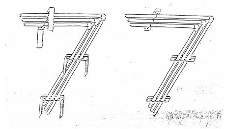
When changing direction in a run of tubing no corner should be unsupported.
