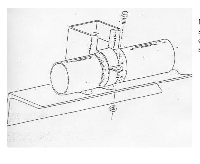
Normally, any straight run of tubing must be supported in at least two locations near each end of the run. Long runs require additional supports.
