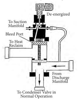
Figure 2-7 Heat Reclaim Valve Normal Operation
