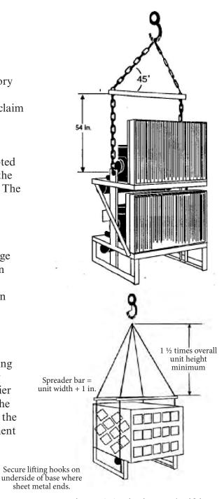
Figure 1-1 Rigging and Lifting
