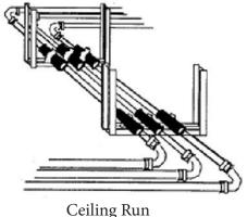
Figure 3-1 Supporting Refrigeration Lines
