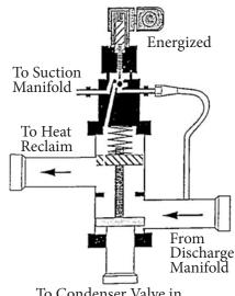
To Condenser Valve in Heat Reclaim Mode
