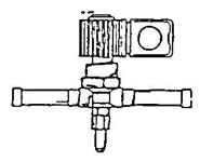
Figure 2-5 Liquid Line Solenoid Valve
