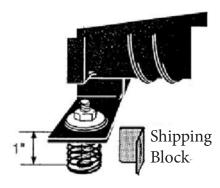
Figure 1-4 Shipping Block Removal
