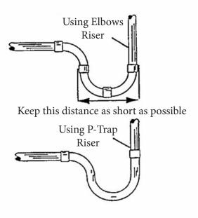
Figure 3-4 P-Trap Construction
