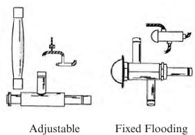
Flooding Valve and Differential Check Valve
