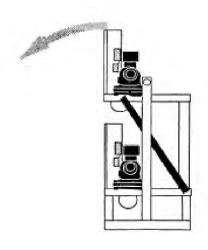
Take appropriate precautions during shipment and moving of unit. Fasten to floor upon final placement.
