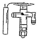
Figure 2-6 Thermostatic Expansion Valve
