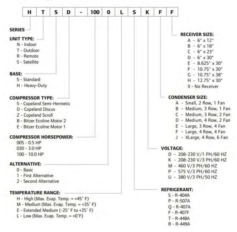
NOTE: Units are ordered refrigerant specific (i.e. "S" for R-404A) but will include other refrigerants that can also be used on the data plate.
