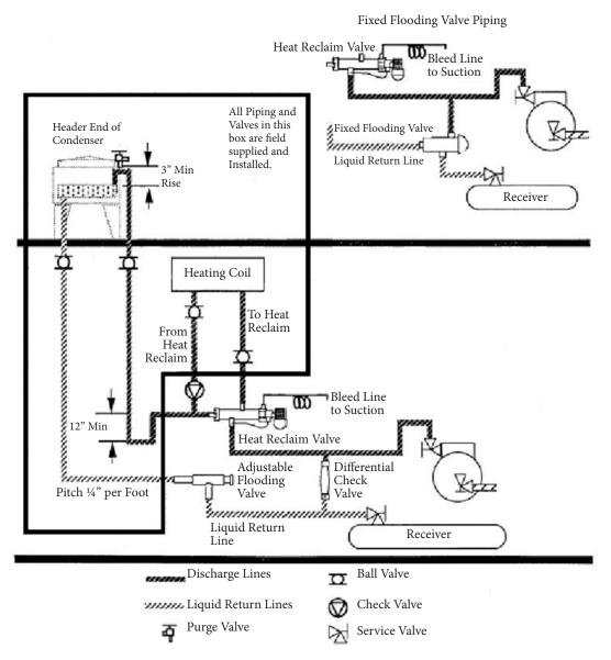
Figure 3-6 Remote Condensing Unit Piping
