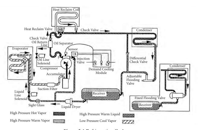
Figure 2-1 Refrigeration Cycle
