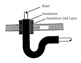
Figure 3-2 Insulating a Riser
