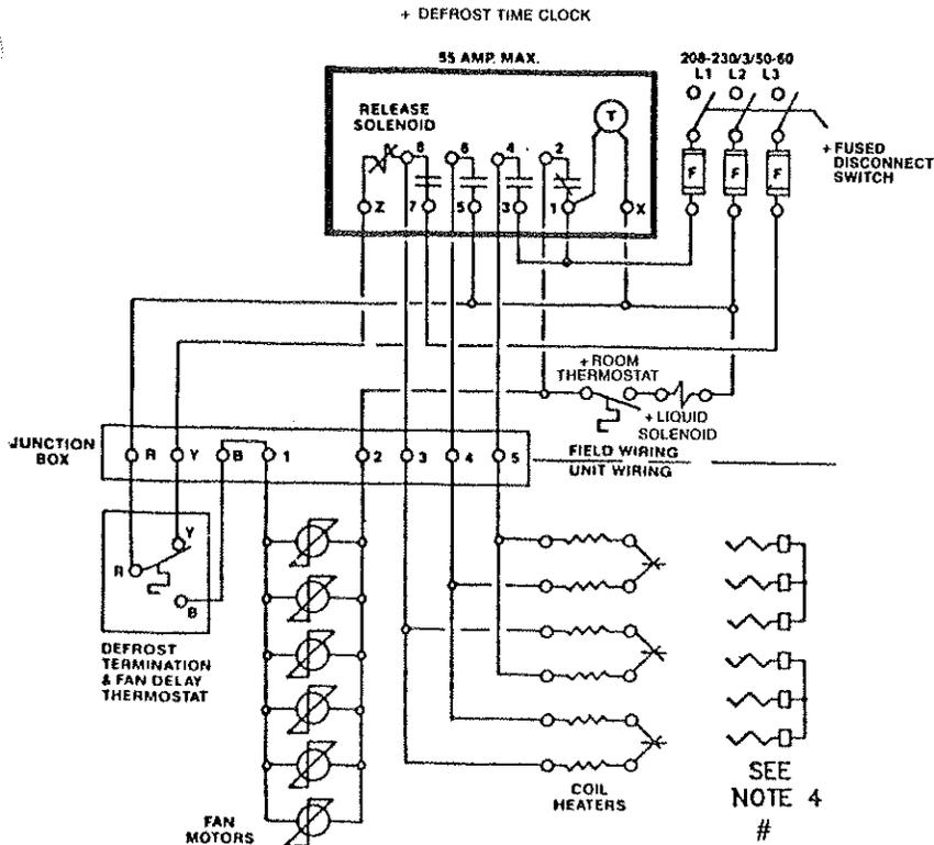
Efficient stainless steel tubular heaters rated for 115 volts, are inserted in fin grooves. Three on the face and three on the coil bottom. Heaters are replaceable from the face or by removing the drain pan. Standard electric defrost configuration is with 208-230/1/50-60 fan motors and heaters wired for 230 volts, single or three phase. If 208 volt or lower power abnormally extends defrost cycles, three phase heaters are easily reconnected in star to obtain 230 volt wattage.
