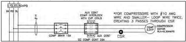
Aux contact wired to 2 terminal pins.
