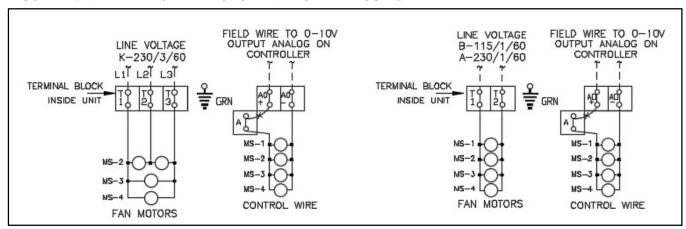
In Case of Variable speed motor coils – the Jumper between terminal A0+ and A should be removed and then and then aux contact from single compressor unit wired in series.
