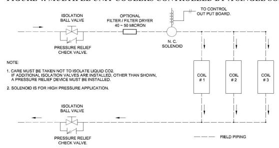
FIGURE 5: MULTIPLE UNIT COOLERS CONTROLLED BY MULTIPLE SOLENOIDS
