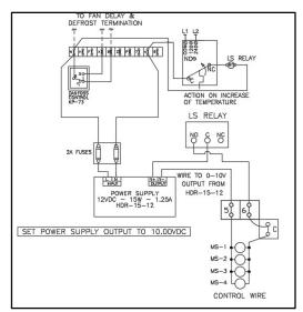
In case of s DUAL SPEED Motor coils with 10V power supply – the Jumper between terminal 6 and C should be removed and then and then aux contact from single compressor unit wired in series. Whenever the compressor contactor energized the Aux contact energizes, and NC contacts changes state to NO, there by OPEN the 10V power supply circuit. So, whenever compressor is ON, fans will never go to low speed mode, even getting signal from Room thermostat or filed controller.
